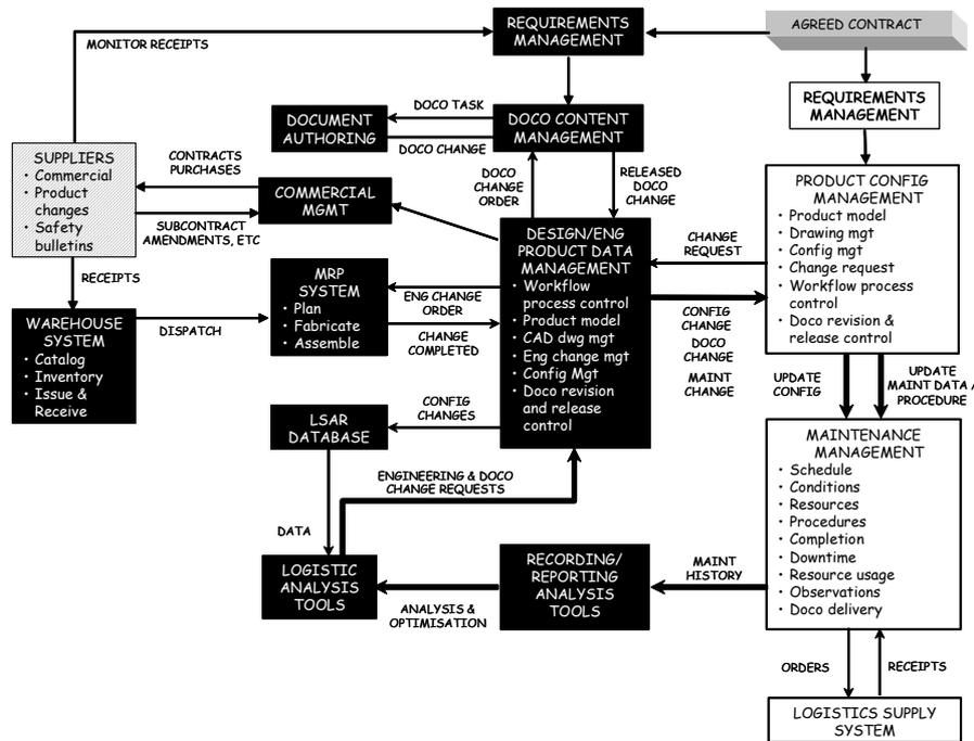
**Figure 5.** Functional components in the PLM paradigm for complex, costly and long-lived engineered product during the "in service support" phase of a project. The client's applications are represented in clear boxes. The prime contractor's applications are shown in black boxes. Note, although they are shown in black here, depending on contractual arrangements, documentation management and logistic analysis for in-service support may be conducted by either the supplier or the client or both.
